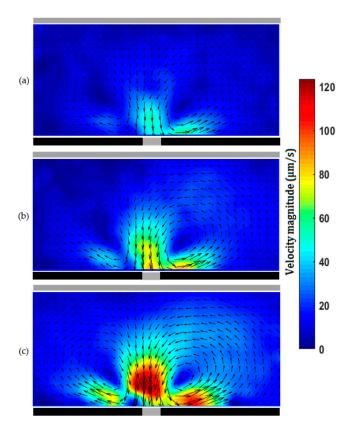
**Figure 4.** Alternating current electroosmosis (ACEO) flow of 1 mM KCl solution between two parallel 0.3 mm pencil-lead electrodes with a gap of 40  $\mu$ m in a microchannel of 0.3 mm diameter. AC voltage of (a) 30  $V_{p-p}$ ; (b) 35  $V_{p-p}$ ; (c) 40  $V_{p-p}$  with a frequency of 50 kHz.
