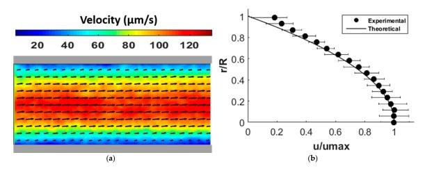
**Figure 2.** (a) Velocity distribution of pressure-driven flow with a volume flow rate of 12  $\mu$ L/h through a microchannel 0.3 mm in diameter; (b) validation of the pressure-driven velocity field in (a).
