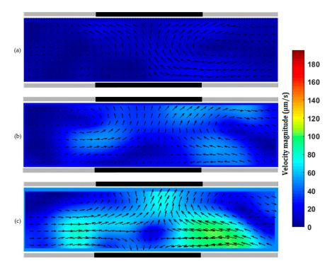
**Figure 5.** ACEO flow of 1 mM KCl solution between two 0.5 mm pencil-lead electrodes facing each other in a microchannel of 0.3 mm diameter. AC voltage of (a) 30  $V_{p-p}$ ; (b) 35  $V_{p-p}$ ; (c) 40  $V_{p-p}$  with a frequency of 50 kHz.
