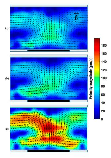
**Figure 3.** Induced-charge electroosmosis (ICEO) flow in front of a 0.5 mm pencil-lead in a channel of 0.5 mm diameter under an applied alternating current (AC) voltage of (a)  $400 \text{ V}_{p-p}$ ; (b)  $450 \text{ V}_{p-p}$ ; (c)  $500 \text{ V}_{p-p}$  with a frequency of 500 Hz between two pencil-lead electrodes positioned about 11 mm apart in reservoirs.
