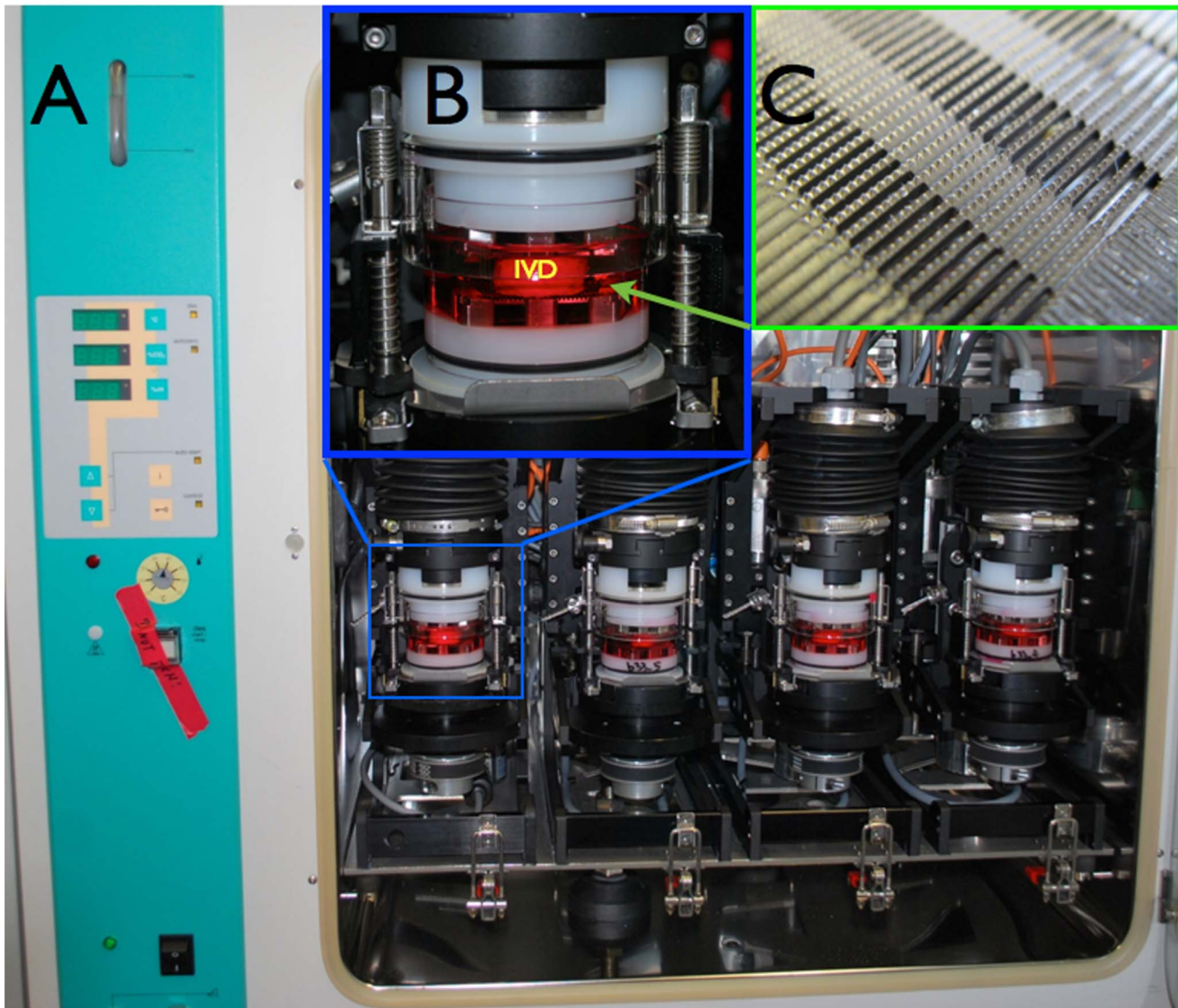
Figure 1. Detailed view of the loading bioreactor and specimen chamber. A) The bioreactor is situated inside a 37°C incubator with 5% CO 2 and 80% humidity. B) The glass walled sample chamber. IVD: intervertebral disc. C) Enlarged view of the titanium plate for holding the samples for rotation movement.
