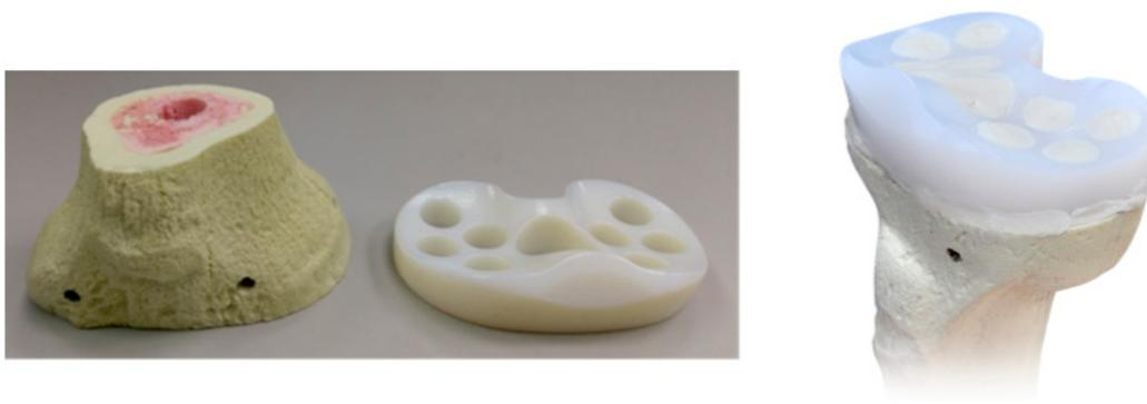
**Figure 5.** Preparation of (top) femoral and (bottom) tibial spacers with sawbones. Spacers are attached onto the resection surface with cement.
