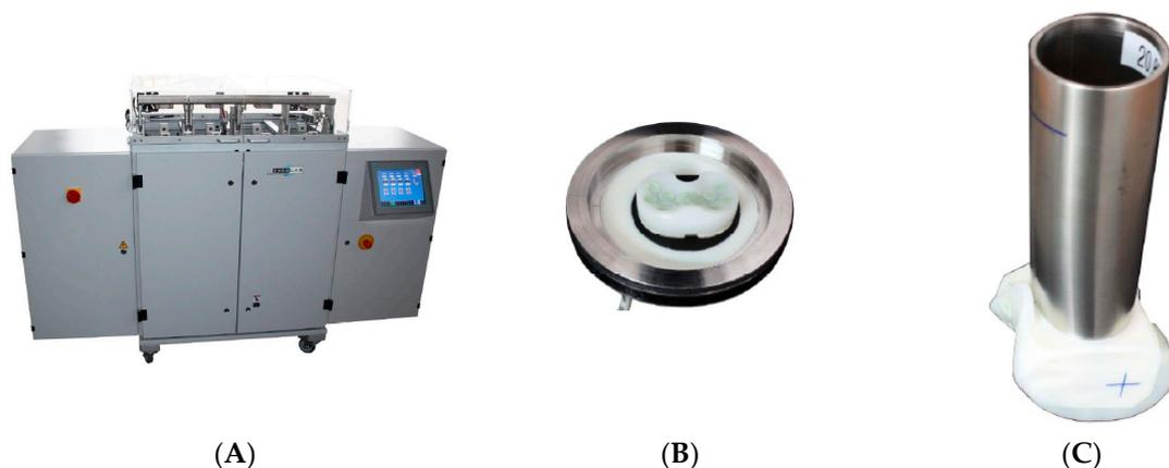
**Figure 7.** (A) The multiple station knee simulator (Endolab), with mounted (B) Tibial spacer and (C) Femoral spacer for wear test.
