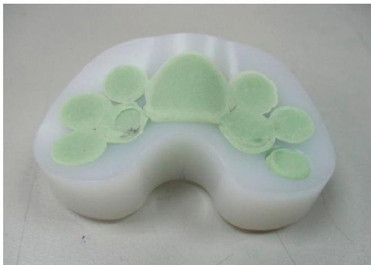
**Figure 9.** Minor cement cracks found on one of the tibial spacers after fatigue testing.
