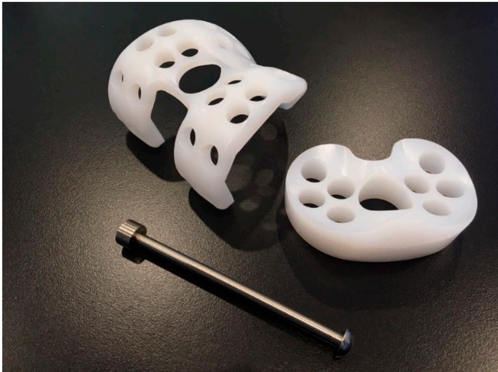
Figure 1. The novel polyethylene-based knee spacer set with canal rod.
