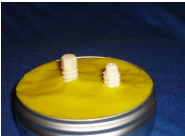
Figure 2 Interference screws derived from bovine bone in polymethyl methacrylate, left BC screw, right Tutofix® screw.
