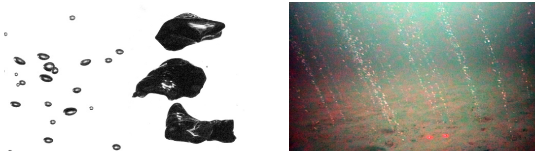
Figure 1. The shape and speed of gas bubbles rising in a liquid depends on the bubbles' volume and surface area and other (physical and chemical) properties of gas and liquid [3]. For instance, air bubbles in water are almost spherical up to millimeter size (small bubbles to the left), become approximately ellipsoidal in the several millimeter range and can be irregularly shaped when much larger. The image to the right shows an area in the North Sea where methane is released from the ocean floor and forms distinct bubble streams. Measuring the flux, the rise speed, and the bubble size distribution is of crucial importance for larger scale ocean and atmosphere models.
