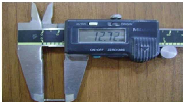
Fig. 2. A digital caliper is used to measure the length of the pins prior to insertion in the mandible.
