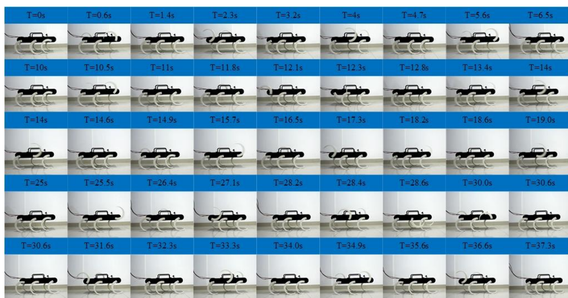
Figure 25. Locomotion experiment of the quadruped, the wave gait, and the mutual transitions.
