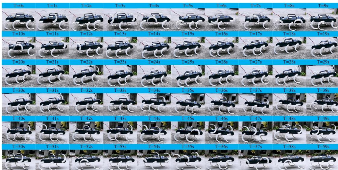
Figure 27. Locomotion and gait transition on uneven ground.
