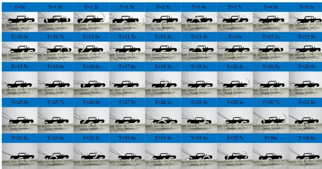
Figure 22. Locomotion experiment of the tripod, the wave gait, and the mutual transitions.
