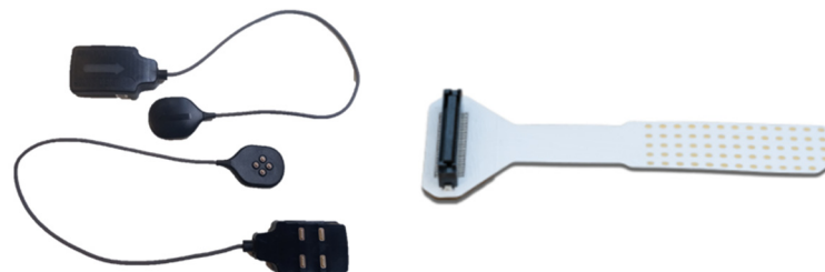
Figure 2. Different sensors used for the decomposition of surface electromyography: Trigno Galileo Sensor of Delsys company and GR04MM1305 of Bioelettronica (left and right panels, respectively). The Bioelettronica sensor image was obtained from the company website ( https://otbioelettronica.it/ , accessed date: 15 July 2021).
