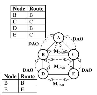
**Figure 2.** Point to Multi-Point (P2MP) and Peer-to-Peer (P2P) Routing Using Multicast Destination Advertisement Object (DAO).
