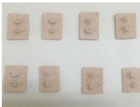
FIGURE 4: Stone dies obtained from impression.
