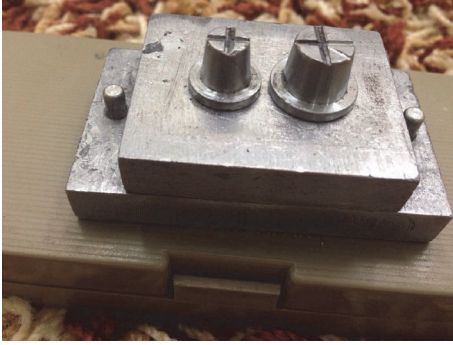
FIGURE 1: Stainless steel master cast used in the study.
