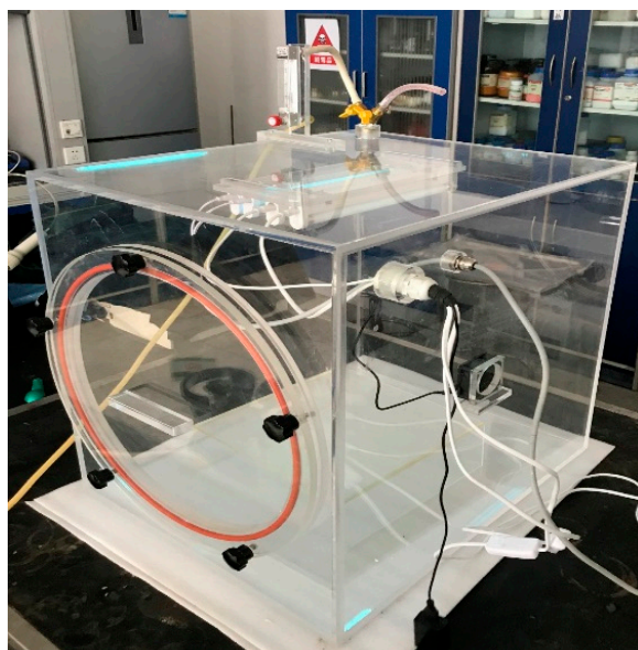
Figure 1. The photocatalytic vehicle exhaust (VE) reaction chamber.
