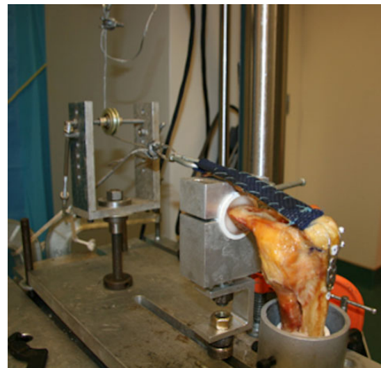
Figure 3. Biomechanical setup of cadaveric specimens in the materials testing system. The proximal end of the humerus was potted in polymethyl methacrylate and flexed to 90°.
