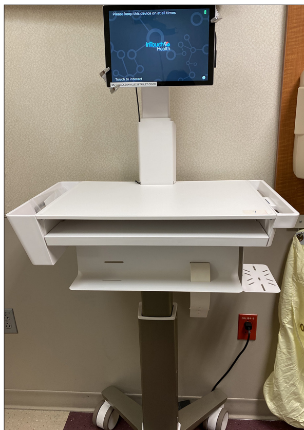
Figure 1. Photo of InTouch Provider® Freestanding Smart Tablet Mobile Workstation: Smart tablet device with audio-video interface is positioned on a mobile workstation on wheels and can be positioned at any location within the Emergency Department.
