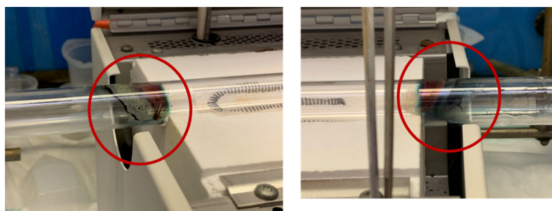
Figure 11. Photographic images taken by authors showing the formation of volatile rhenium species on both ends of the quartz tube following the thermal threat of \text{C}_6\text{H}_6\text{N}_3[\text{ReO}_4] at 700 °C in air.
