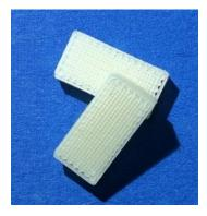
**Figure 2.** Picture of printed objects  $(3 \times 15 \times 7.5 \text{ mm})$  using in-house-produced filaments based on EC and HPMC for the evaluation of uniformity of mass according to Ph.Eur. 2.9.5.
