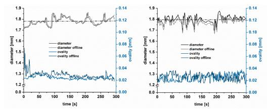
**Figure 3.** Inline- and offline-determined diameter and ovality ( $\Delta \emptyset_{max/min}$ ) as a function of time (1 Hz) for each applied PFR = 5 g/min (left); 10 g/min (right). The dashed line marks the mean value of the inline-determined diameter.
