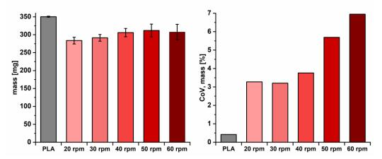
**Figure 9.** Mass of printed objects (n = 20, mean  $\pm$  s) of filaments produced with different screw speeds compared to commercial PLA filaments (**left**) and CoV<sub>mass</sub> (**right**).
