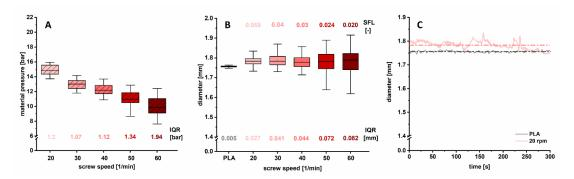
**Figure 6.** Boxplot of material pressure (**A**) and filament diameter (**B**) for different applied screw speeds during extrusion (1 Hz; n > 290). Resulting SFL and IQRs (box width) are indicated. Inline determined diameter as function of time for commercial PLA filament compared to produced filament with 20 rpm (**C**); dashed lines mark the mean value.
