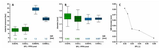
**Figure 7.** Boxplots of inline determined material pressure (**A**) and diameter (**B**) during HME for two different applied SFL on a high (10 g/min, HL) and low (5 g/min, LL) PFR-level, respectively (1 Hz, n > 290). IQRs of pressure and diameter are indicated. (**C**) displays diameter IQR as function of different applied screw speeds (n > 290).
