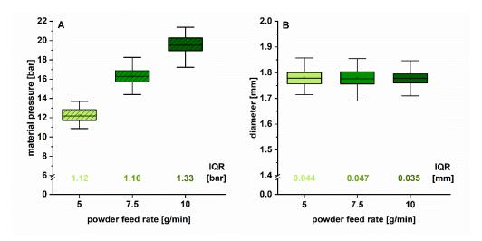
**Figure 5.** Boxplot of inline measured material pressure at the die (**A**) and filament diameter (**B**) (1 Hz, n > 294) for different applied PFR. The respective IQRs (box width) are indicated.
