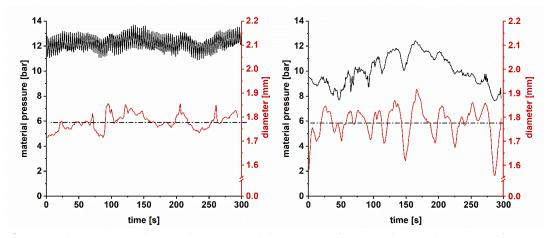
**Figure 4.** Inline determined material pressure and diameter as a function of time, where a PFR of 5 g/min and a screw speed of 40 rpm (**left**) or 60 rpm (**right**) were applied. The dashed lines mark the mean diameter.
