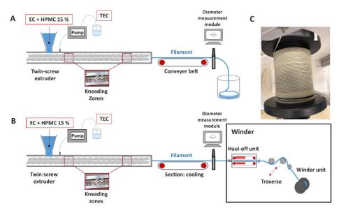
**Figure 1.** HME setup for filament production before (**A**) and after (**B**) optimization by implementing a winder. Subfigure (**C**) displays an exemplary winding process in the winder unit.
