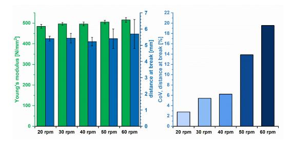
**Figure 8.** Determined YM and distance at break of filaments produced at different screw speeds (mean  $\pm$  CI, *n* = 6 ( $\alpha$  = 0.05), **left**) and the CoV<sub>distance at break</sub> related to the applied screw speed (**right**).
