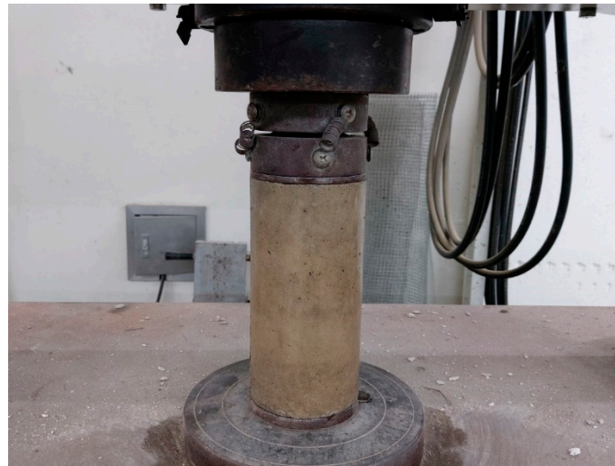
Figure 2. Compressive strength test configuration.
