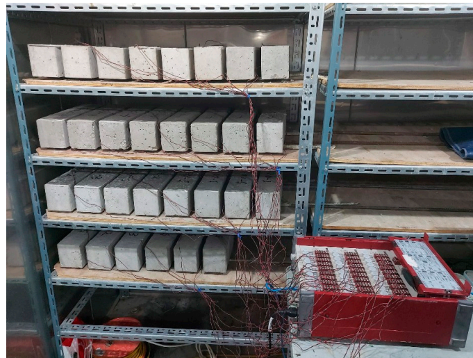
Figure 4. Drying shrinkage test.
