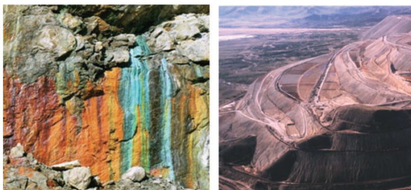
Fig. 1. (Left) Natural leaching of the mineral chalcopyrite (CuFeS 2 ), which then is precipitated as a mixture of chrysocolla (light blue copper silicate) and malachite (green copper-carbonate-sulfate). The rust-brown colour is a precipitation of iron (oxide/hydroxide), another product of the chalcopyrite leaching reaction. Courtesy of Torbjörn Kjellsson (Kjellsson, 2002). (Right) Large dump-leaching facility at a copper mine operation near Salt Lake City, Utah ( http://www.personal.psu.edu/faculty/j/e/jel5/biofilms/leaching.html ).
