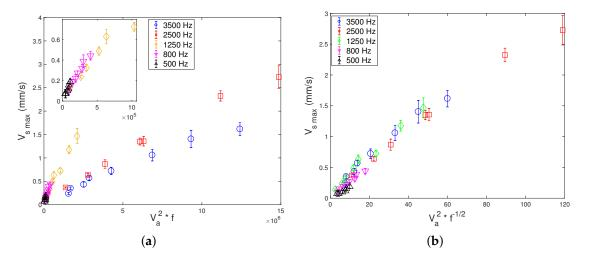
**Figure 11.** Attempts of data rescalling for  $V_{s \max}$  (**a**) versus  $V_a^2 \times f$  (insert shows data in the lowest range of  $V_a^2$ ) and (**b**) versus  $V_a^2 \times f^{-1/2}$  showing a fair collapse of data.
