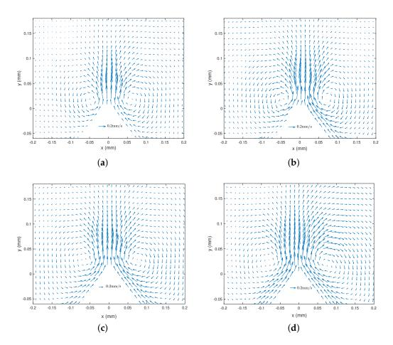
**Figure 7.** Streaming velocity field  $V_s(x, y)$  from PIV measurements, with different excitation frequencies  $v = 4.32 \text{ mm}^2/\text{s}$  (Fluid 3) and  $V_a = 22.4 \text{ mm/s}$ . (a) f = 3500 Hz, (b) f = 2500 Hz, (c) f = 1250 Hz, (d) f = 800 Hz. Scales are the same for the four cases.
