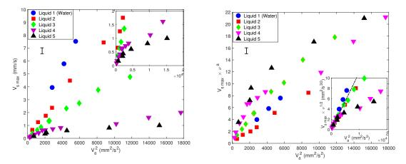
**Figure 6.** Left —Maximal streaming velocity  $V_{s max}$  versus the square of the acoustic forcing velocity  $V_a^2$ , for different liquid viscosities  $\nu$ , indicated in Table 2. Right—Quantity  $V_{s max} \times \nu^{-a}$ , with a = -0.9. Inset  $V_{s max} \times \nu^{1/2}$ . All measurements were obtained at f = 2500 Hz. The averaged typical error bar is indicated.
