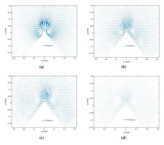
**Figure 3.** Streaming velocity field  $V_s(x, y)$  from PIV measurements, with different liquid viscosities. f = 2500 Hz and  $V_a = 35$  mm/s. (a)  $\nu = 1.158$  mm<sup>2</sup>/s, (b)  $\nu = 4.32$  mm<sup>2</sup>/s, (c)  $\nu = 13.75$  mm<sup>2</sup>/s, (d)  $\nu = 29.44$  mm<sup>2</sup>/s. Scales are the same for the four cases.
