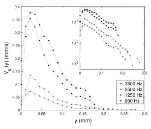
**Figure 9.** Streaming velocity profile along vertical direction  $V_s(y)$ , for four different frequencies. Liquid viscosity  $\nu = 4.32 \text{ mm}^2/\text{s}$  and  $V_a = 22 \text{ mm/s}$ . The inset plots the same data in Lin-log axes.
