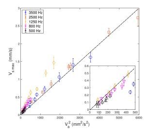
**Figure 10.** Maximal streaming velocity  $V_{s max}$  versus  $V_a^2$ , for different *f* and the same viscosity  $\nu = 4.32 \text{ mm}^2/\text{s}$ . The dashed-dotted line suggests a linear relationship, with a prefactor  $\theta = 5 \times 10^{-4} \text{ s/mm}$ . The inset represents a magnified view of the plot for the lowest values of  $V_a^2$ , suggesting a linear scaling with a prefactor  $\theta = 0.0011 \text{ s/mm}$ .
