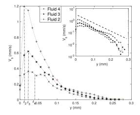
**Figure 5.** Streaming velocity profile along vertical direction  $V_s(y)$ , for three different viscosities (Fluids 2, 3 and 4 with  $\nu$  respectively equal to 1.158, 4.32 and 13.75 mm<sup>2</sup>/s). The operation condition is at frequency f= 2500 Hz and acoustic velocity  $V_a$  = 35 mm/s. Additionally labelled are the values of the VBL thickness for the three fluids  $\delta_2$ ,  $\delta_3$  and  $\delta_4$ . The inset plots the same data in Lin-log axes.
