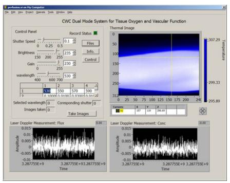
**Figure 2. Software interface for the CWC system.** The software interface was programmed in the Labview environment. On the top left of the interface is the control panel for hardware configuration and system calibration. On the right of the interface is the real-time display of the tissue temperature map acquired by the infrared camera. On the bottom of the interface are laser Doppler measurements of skin tissue perfusion.
