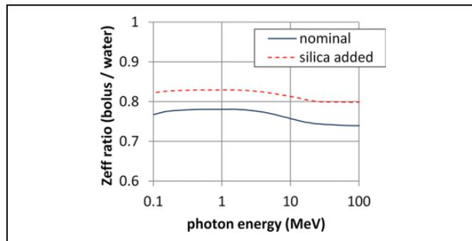
**Figure 4.** Effective atomic number as a function of photon energy for the finalist bolus material (15% polymer B prior to silica) with and without added silica (9% by weight) to achieve equal density to water.
