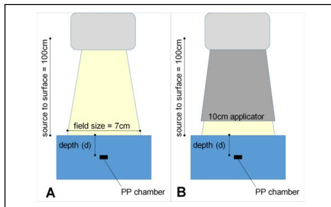
**Figure 1.** Experimental setup for measurement of percent depth dose in solid water and polymeric gel material for photons (A) and electrons (B).
