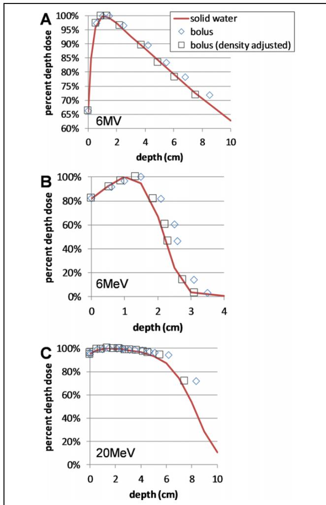
**Figure 5.** Percent depth dose measured through selected polymeric gel material (15% polymer B, no silica) compared to water equivalent plastic phantom. The dose curves coincide after scaling  $x$ -axis for density for 6MV photons (A), 6MeV electrons (B), and 20MeV electrons (C).
