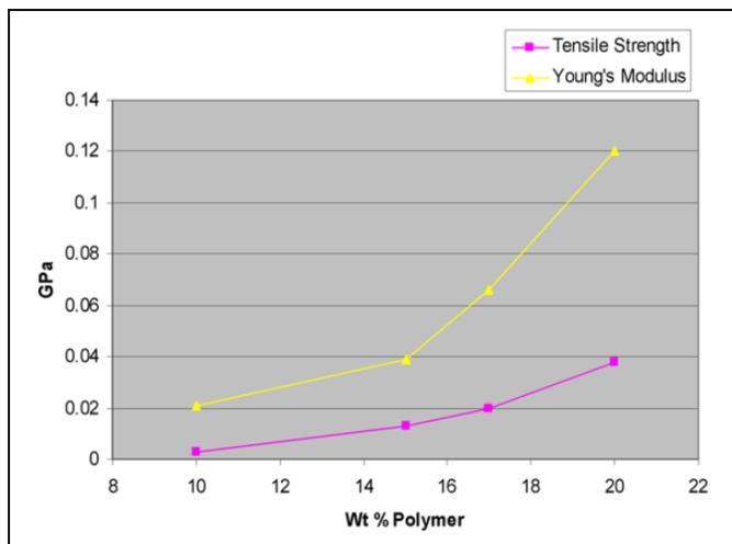
**Figure 3.** Tensile strength and Young modulus as a function of percent weight of polymer B. Mechanical properties of the bolus material can be optimized by adjusting the polymer content.
