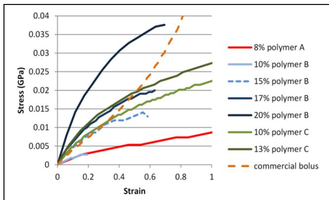
**Figure 2.** Stress–strain curve measured for polymeric gel combinations, compared to a commercial bolus material. The polymeric gel with 15% of polymer B was selected for further characterization.
