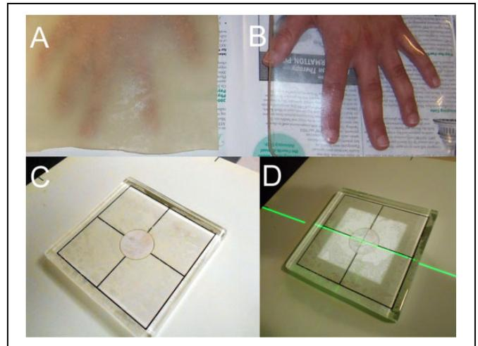
**Figure 6.** Visibility through commercial bolus (A) and polymeric gel (B-D) materials. Localization marks and the light field could be easily visualized on the surface through the polymeric gel material.
