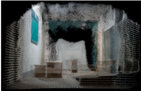
Fig. 4. Sample of filtered 3D dense map of experimental corridor workspace.
