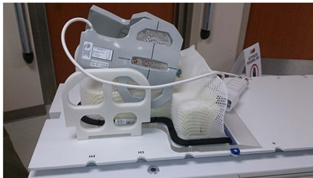
Figure 1. Patient immobilization device and magnetic resonance imaging (MRI) coil arrangement. Imaging patients while immobilized in the position in which they would receive radiation treatment drastically reduces motion artifact, enabling the acquisition of high-quality chemical exchange saturation transfer (CEST) and other MR images.
