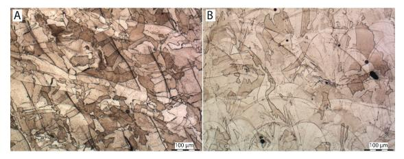
**Figure 4.** Microstructure of sample HT1: (**A**) in direction parallel with direction of application of individual layers, (**B**) in direction perpendicular to direction of application of individual layers (etched in Villella).
