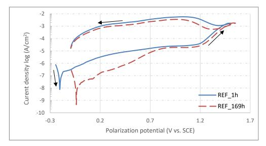
**Figure 10.** Semilogarithmic polarization curves for sample REF after 1 and 169 h exposition in physiological solution.
