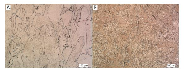
**Figure 5.** Microstructure of sample HT2: (**A**) in direction parallel with direction of application of individual layers, (**B**) in direction perpendicular to direction of application of individual layers (etched in Villella).
