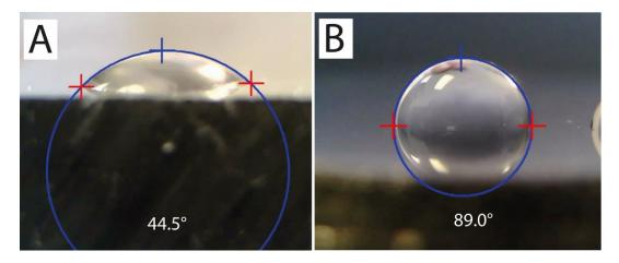
**Figure 15. A**-Droplet on the surface of an REF sample prepared by SLM; **B**-droplet on the surface of a wrought sample.
