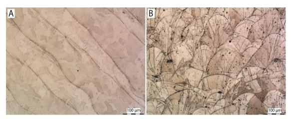
**Figure 6.** Microstructure of sample REF: (**A**) in direction parallel with direction of application of individual layers, (**B**) in direction perpendicular to direction of application of individual layers (etched in Villella).
