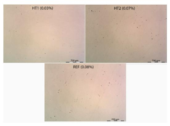
Figure 2. Macroimage of surfaces of HT1, HT2 and REF samples used for porosity determination.
