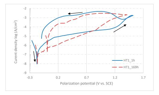
**Figure 8.** Semilogarithmic polarization curves for sample HT1 after 1 and 169 h of exposition in physiological solution.
