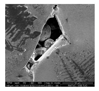
Figure 3. Microstructure of pores in detail, showing nonmelted round particles inside.
