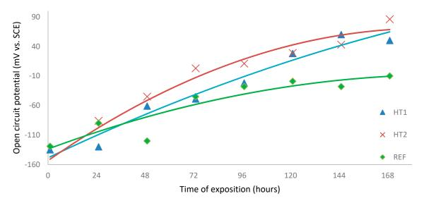
Figure 7. Chart of OCP evolution in 169 hours exposition for each sample.
