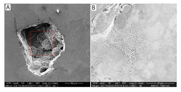
**Figure 11. A**-Corrosion pit with rough inner surface and traces of non-welded particles; **B**-honeycomb-like structure on the exposed surface as a sign of selective corrosion.
