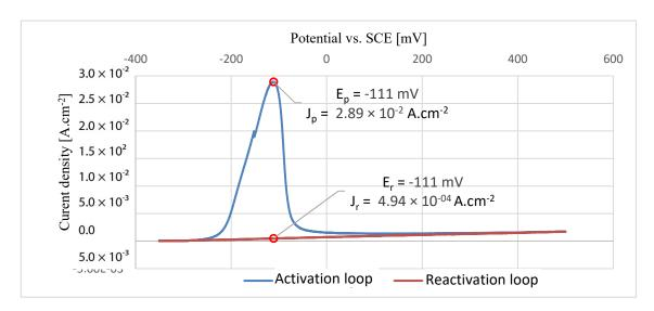
Figure 14. EPR-DL curve for REF sample.
