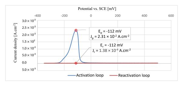
Figure 12. EPR-DL curve for HT1 sample.
