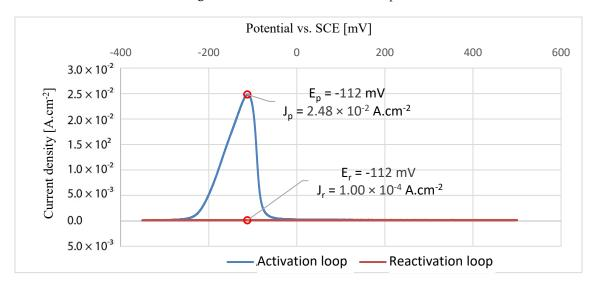
Figure 13. EPR-DL curve for HT2 sample.
