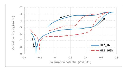
**Figure 9.** Semilogarithmic polarization curves for sample HT2 after 1 and 169 h exposition in physiological solution.
