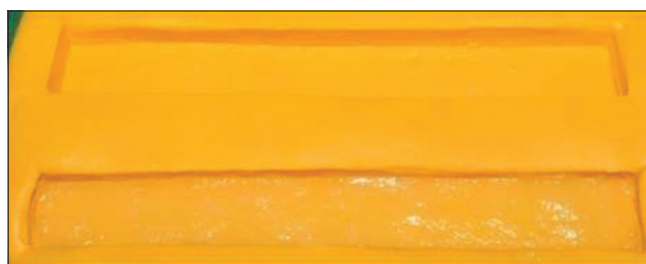
Figure 2: Fiber-reinforced composite resin dispensed into putty addition silicone mold
