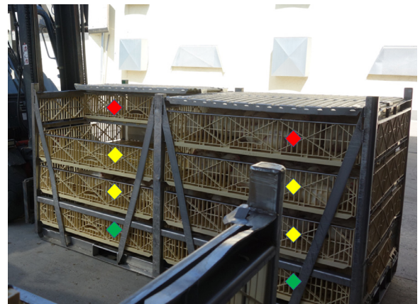
Figure 2. Metal container of the type GP live bird container supply system from the company Marel (Austurhraun 9, Gardabaer, IS-210 Iceland). The container consisted of a metal frame with a total of 8 crates, divided into 2 sides (left and right) with 1 low (green), 2 middle (yellow), and 1 high crate (red) on each side; each crate is opened and closed manually during loading.
