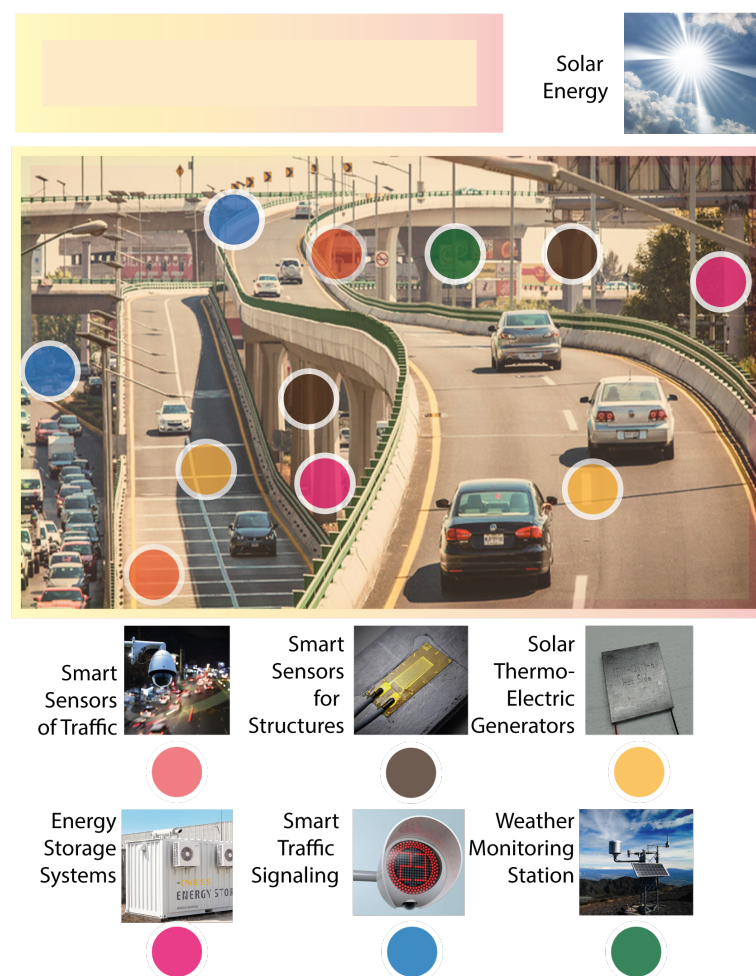
Figure 1. Smart system example for the management of traffic using solar thermoelectric generation in urban highways.
