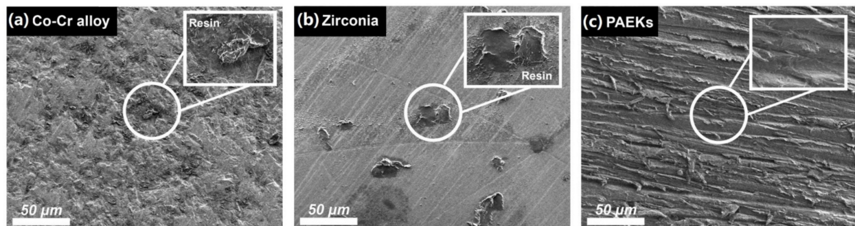
Figure 4. The representative debonded surface morphologies of each group of materials. The FE-SEM image (the magnification was 500 \times and the scale bar was 50 \mu m) of (a) the Co-Cr alloy (AP group, pretreatment with both sandblast and primer), (b) zirconia-based ceramic (PR group, primer pretreatment by priming with primer), and (c) (Poly)aryl-ether-ketone materials (PAEKs) (AP group). Residual denture acrylic debris was found in the Co-Cr alloy and zirconia-based ceramic, as shown in the magnified pictures, while the debonded surfaces of the PAEKs shown no residuals.
