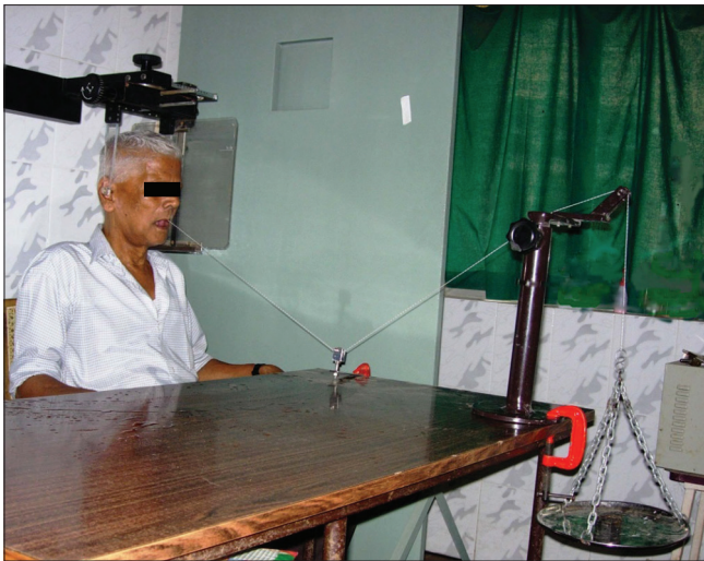
Figure 6: Test with Pulley suspended retention apparatus
