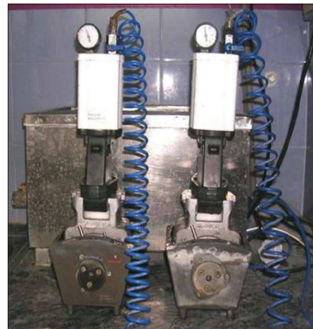
Figure 3: Injection of resin into flask under hydraulic pressure
