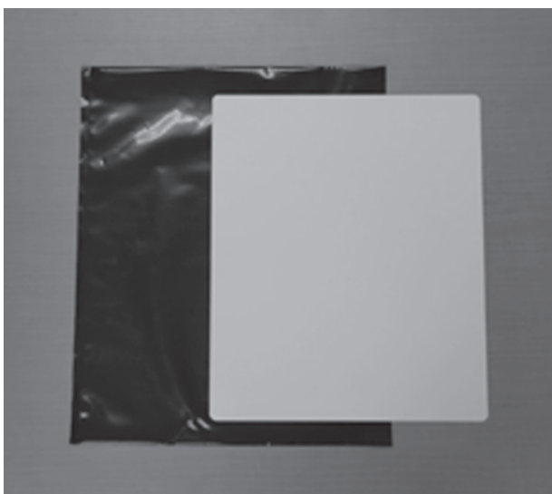
Fig. 1. The appearance of cassetteless method of a imaging plate and a commercially available hard black plastic bag.
