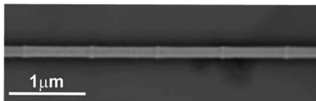
Figure 1. Scanning electron microscopy image of an individual bamboo-like nanowire.
