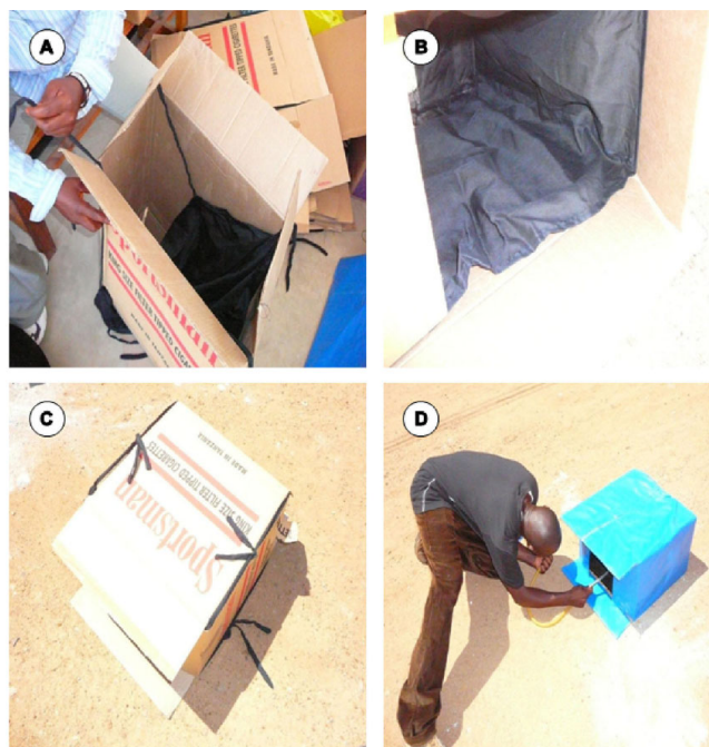
Figure 1 Photographs of the standardized resting boxes (SRB) used in this study. Panels A and B illustrate how the boxes are made, panel C demonstrates the way to install them, and panel D demonstrates how to recover resting mosquitoes.
