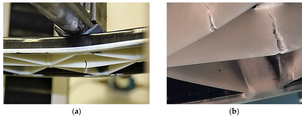
Figure 6. Three-point flexural test of the PP/GF60 and PP/GF30 hybrid injection molded thermoplastic composite test structure: (a) test set-up and (b) failure of ribs as a result of the bending load.
