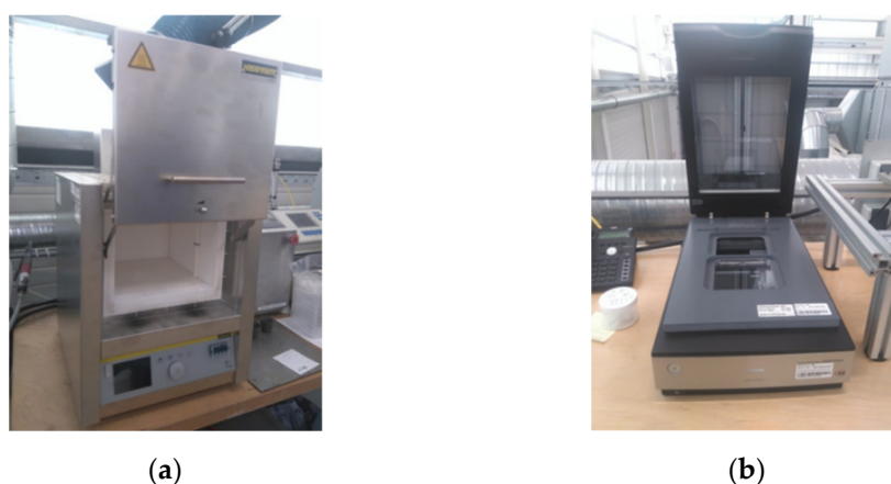
Figure 3. Experimental equipment used for fiber length analysis of the PP/GF30 short fiber-reinforced thermoplastic composite: (a) electric furnace and (b) photo scanner.
