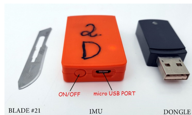
Figure 3. The external appearance of an IMU and the wireless connection dongle.
