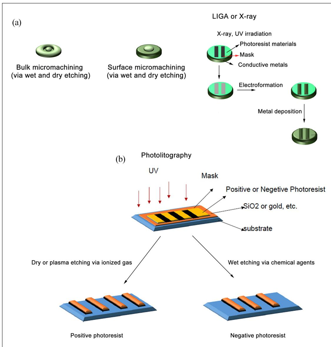
**Figure 2.** (a) MN fabrication methods are a subset of micro-electro-mechanical fabrication processes that diverged into three major groups: bulk micromachining, surface micromachining, and LIGA. (b) Photolithography process is one of the methods to the pattern desired figures on biomaterials, subsequently creating the 3D shape via wet or dry etching.
