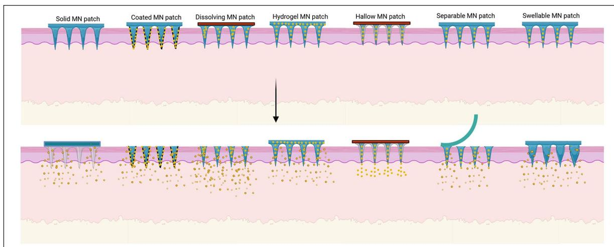
**Figure 4.** Types of MNs with different releasing mechanisms.
