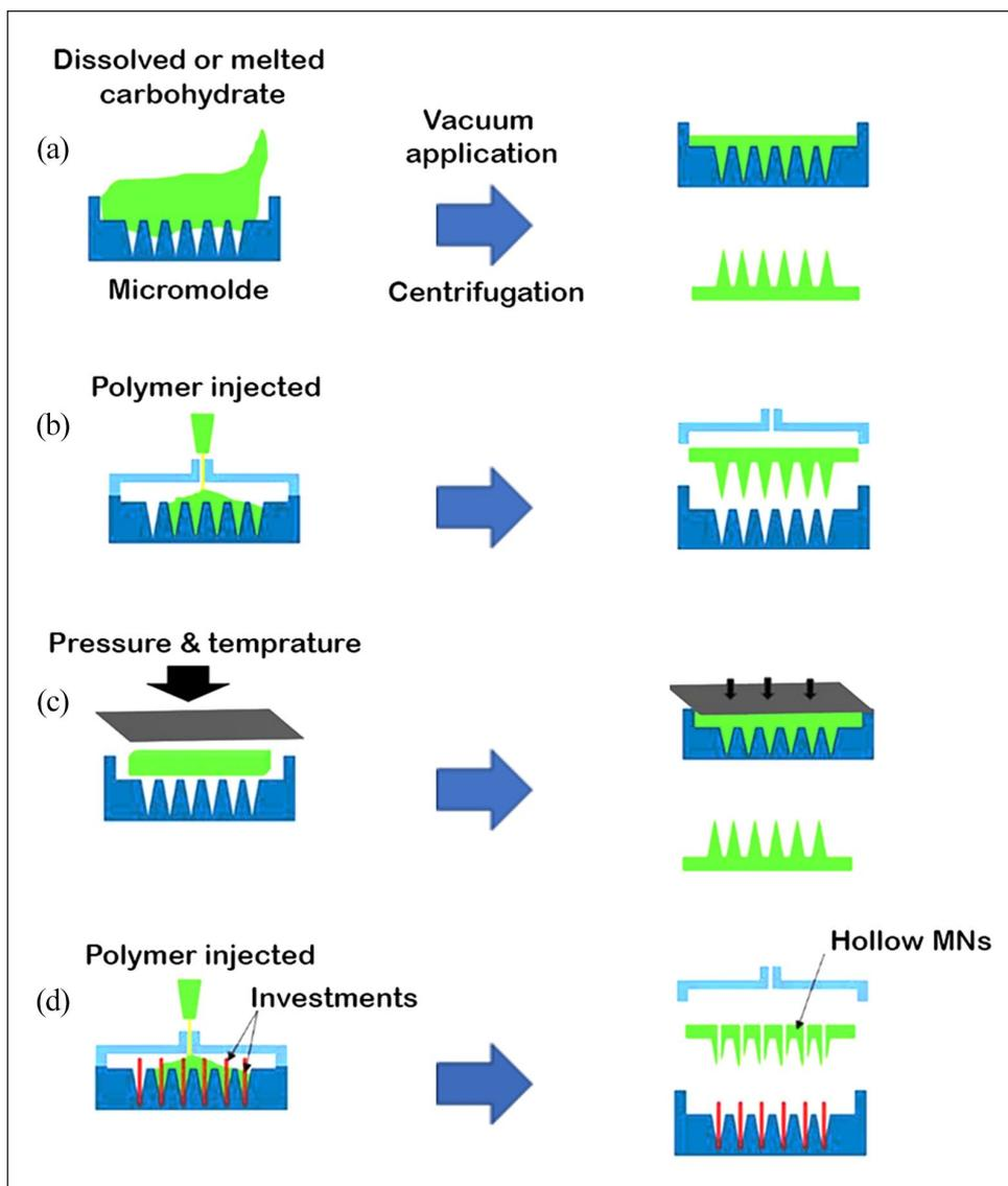
**Figure 3.** Several micromolding-based MN fabrication techniques: (a) micromolding, (b) injection molding, (c) hot embossing, and (d) investment molding.
