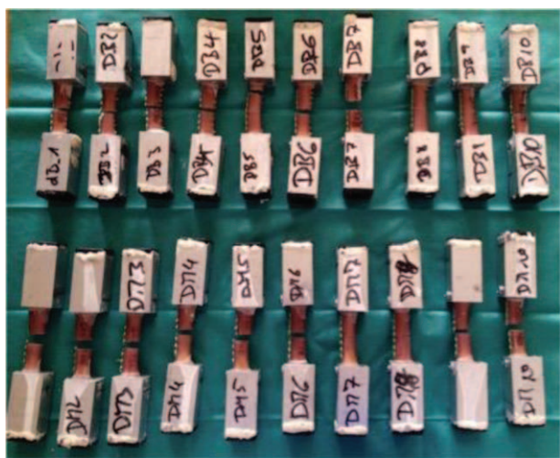
Figure 6. All the constructs that failed in the cycling loading test broke at the osteotomy point.
