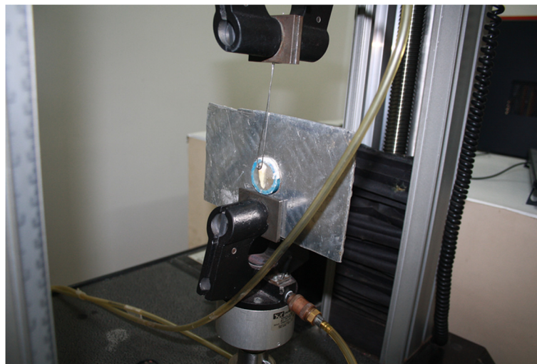
Figure 1 Specimens were mounted on jig secured to the lower jaw of universal testing machine. A 0.03-in wire was attached to the upper jaw which applied shear forces at a crosshead speed of 3 mm/min.
