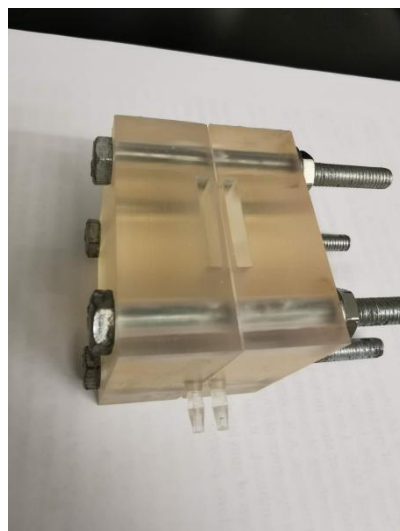
Supplementary Fig. 24 Photograph of the experimental setup device for osmotic energy conversion performance test. The device is connected to the external detection equipment for collecting output current and voltage.
