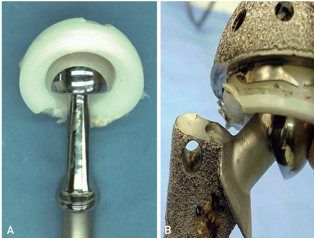
Fig. 11. (A, B) Retrieved acetabular and femoral components from a 43-year-old male patient revealing polyethylene liner damage by impingement between the rim of polyethylene liner and neck of the femoral stem.
