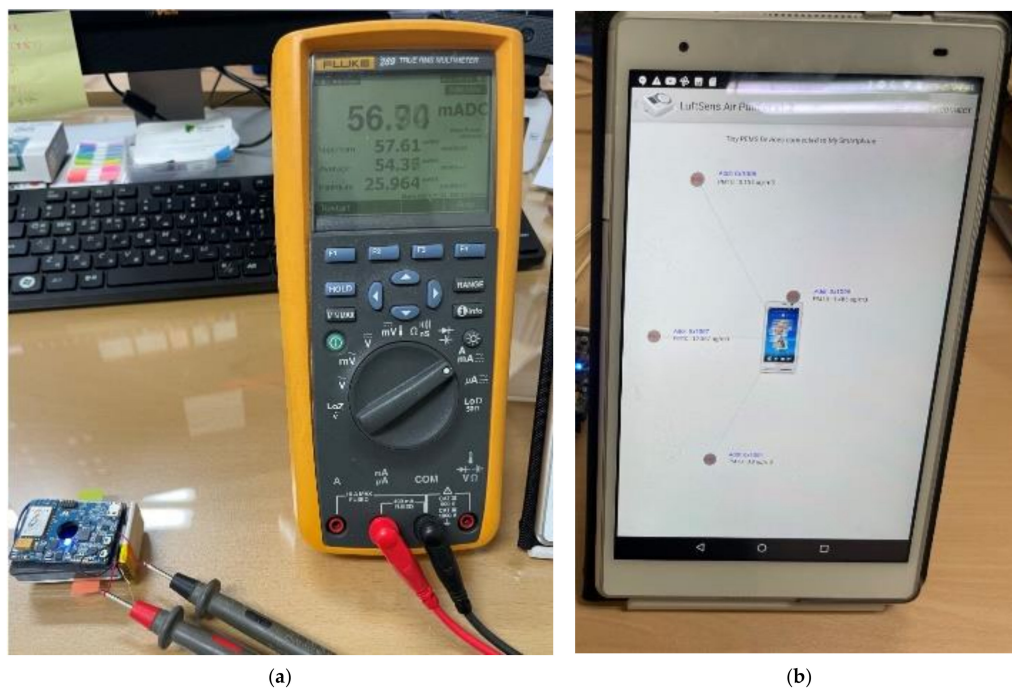
Figure 16. Power consumption and GUI of the smartphone: (a) environment for power consumption measurement (b) Smartphone GUI.
