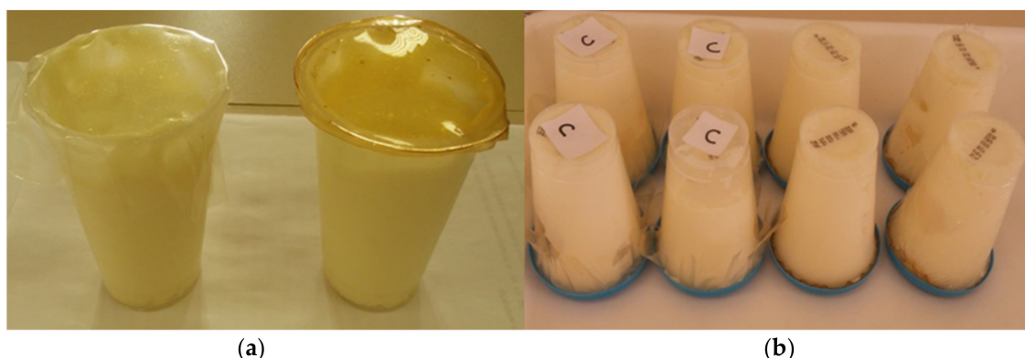
Figure 1. Application of active bioplastic film on curd cheese. (a) Replacement of the aluminum membrane for the control film and extract; (b) Inverted product storage so that it comes in direct contact with the film.
