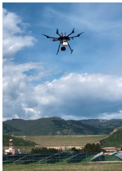
Figure 4. Photograph of sUAS in the air with integrated methane sensor.
