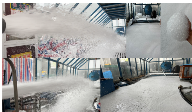
Figure 13. Foaming effect of gas-liquid coaxial and Venturi tube foam generator (photograph courtesy of author).
