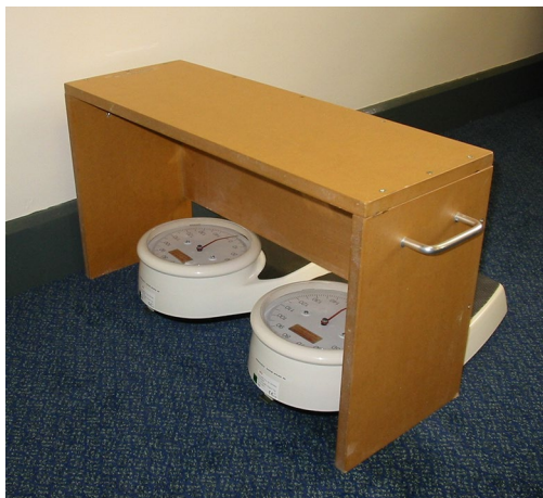
Fig. 1 Two scales are placed on the floor with dials concealed from the subject
