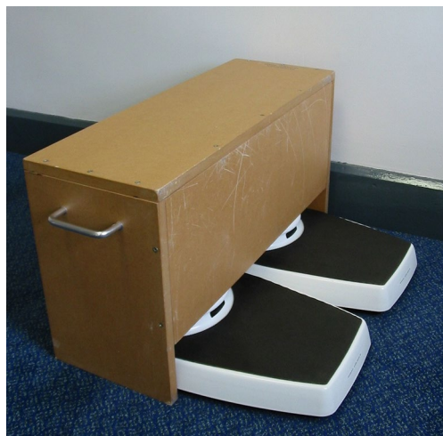
Fig. 2 Two scales are placed on the floor with dials concealed from the subject
