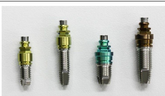
Figure 2 The implants in this study. Two kinds of diameters (3.8 mm, 5.0 mm) and two kinds of lengths (7.0 mm, 12.0 mm) having a general threadlike shape with a mechanically polished surface.
