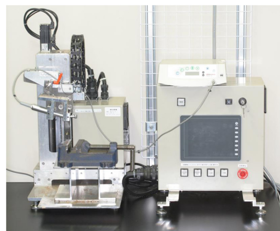
Figure 3 The special implant cavity-forming device. This device is able to adjust the up-and-down movement speed and the rotation speed of the drill.
