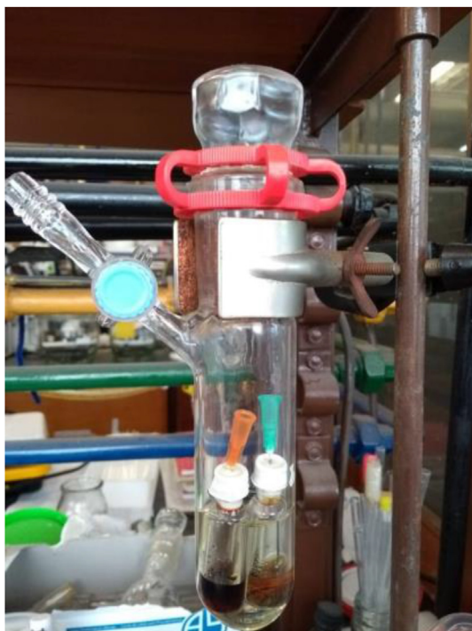
Figure 11. Crystallization setup for (\text{BTMA})_2\text{Mg}[\text{Fe}^{\text{II}}(\text{TPPS}) (\text{NO}^*)] under argon. Initially, a deoxygenated aqueous saturated solution of the complex is placed in the vials. Degassed acetone (approximately 10–15 ml) is placed inside the Schlenk tube, surrounding the vials. Needles are punctured through the vials' septa to allow slow vapor diffusion.
