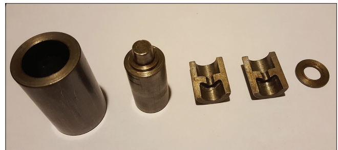
Figure 2: Disassembled stainless steel master die
