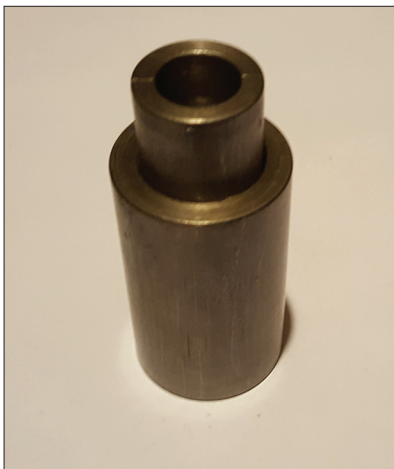
Figure 1: Stainless steel master die used in the study
