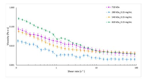
**Figure 1.** Equilibrium flow curves of 0.15~mg/mL HA aqueous solutions by HA with different molecular weights, namely 280~kDa (blue dotted line), 540~kDa (orange dotted line), 710~kDa (violet dotted line), and 820~kDa (green dotted line).
