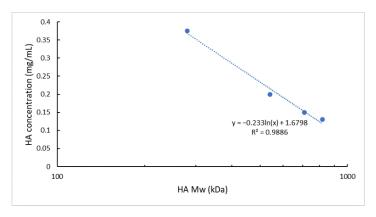
**Figure 3.** Interpolation of the ln (HA Mw) vs. HA solution concentration. Experimental points correspond to 280, 540, 710, and 820 kDa Mw HA and the relative HA solution concentrations used in the NPs microfluidics-based preparation method.
