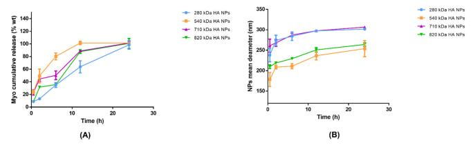
**Figure 5.** (**A**) Myo in vitro release from Myo280\_20 (blue line), Myo540\_15 (orange line), Myo710\_15 (violet line), and Myo820\_20 (green line) in 72 h: Myo-HA NPs were incubated in 0.01 M PBS pH 7.4 at 37 °C to best simulate the physiologic environment. Results represent the mean  $\pm$  SD; n = 3 independent batches. (**B**) Swelling phenomena representation: Myo280\_20 (blue line), Myo540\_15 (orange line), Myo710\_15 (violet line), and Myo820\_20 (green line).
