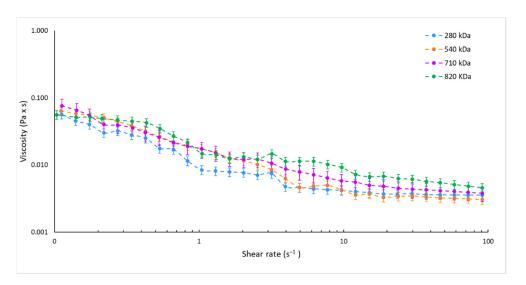
**Figure 2.** Equilibrium flow curves of HA solutions at 0.325, 0.200, 0.150, and 0.130 mg/mL by using HA with Mw of 280 kDa (blue dotted line), 540 kDa (orange dotted line), 710 kDa (violet dotted line), and 820 kDa (green dotted line), respectively.
