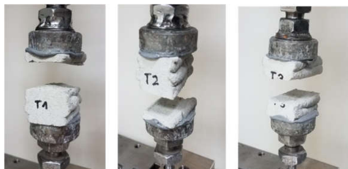
Figure 12. Samples after the direct tensile strength test and the mode of rupture of samples T1, T2, and T3.
