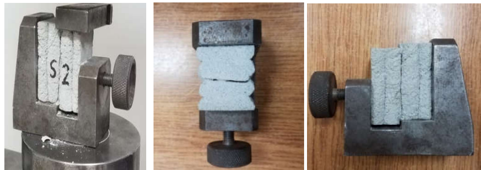
Figure 16. The failure mode of samples after the shear strength test.
