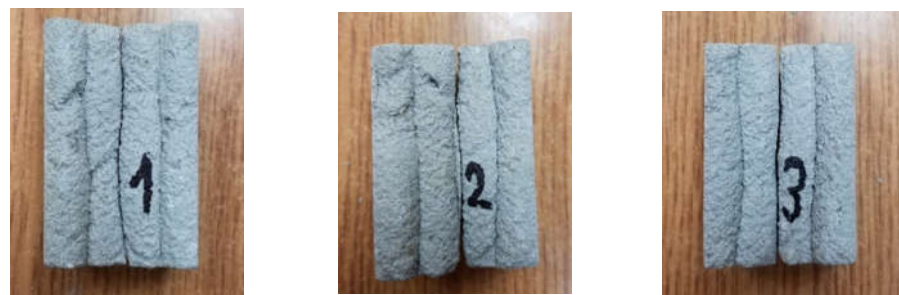
Figure 14. The failure mode of the samples after the splitting test.
