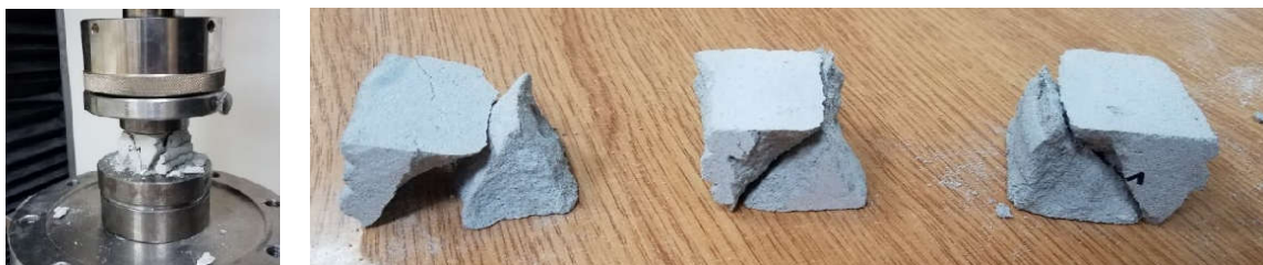
Figure 10. Representative example of samples after the compressive strength test and the mode of rupture of samples, from the right: C1, C2, and C3.
