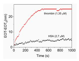
**Figure 6.** Optical response (EOT-EOT<sub>0</sub>) after the exposure of TBA aptamer to 1.35  $\mu$ M of thrombin (red line) and to 2.7  $\mu$ g/mL of HSA (black line).
