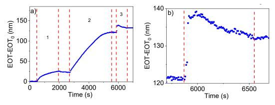
**Figure 4.** (a) Registered change in EOT as a function of time during NAA surface functionalization: (1) sulfo-NHS-biotin, (2) streptavidin, (3) trombin-binding-aptamer (TBA). (b) A close-up of the EOT variation with time of the step 3 of the experiment in Figure 4a.
