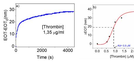
Figure 5. Study of thrombin detection. (a) Variation of EOT with time for one of the experiments performed for thrombin detection of 1.35 μM. (b) Absolute change in ΔΕΟΤ at different concentrations of thrombin. Red line represents a calibration curve by fitting with Boltzmann equation.
