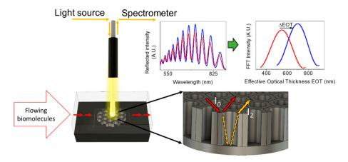
Figure 2. Explicative scheme of the Reflectometric Interference Spectroscopy system (RIfS).
