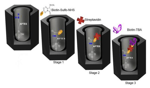
Figure 3. Schematics of aptamer immobilization into NAA pores.
