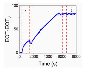
**Figure 7.** EOT evolution during the sulfo-NHS-biotin (1), streptavidin (2) and thrombin infiltration (3) without TBA.
