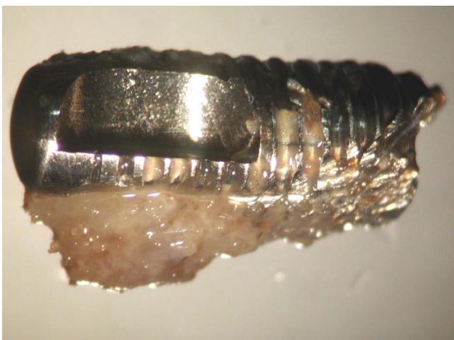
Figure 3 Stereomicroscope imaging showing well-osseointegrated fractured implant.
